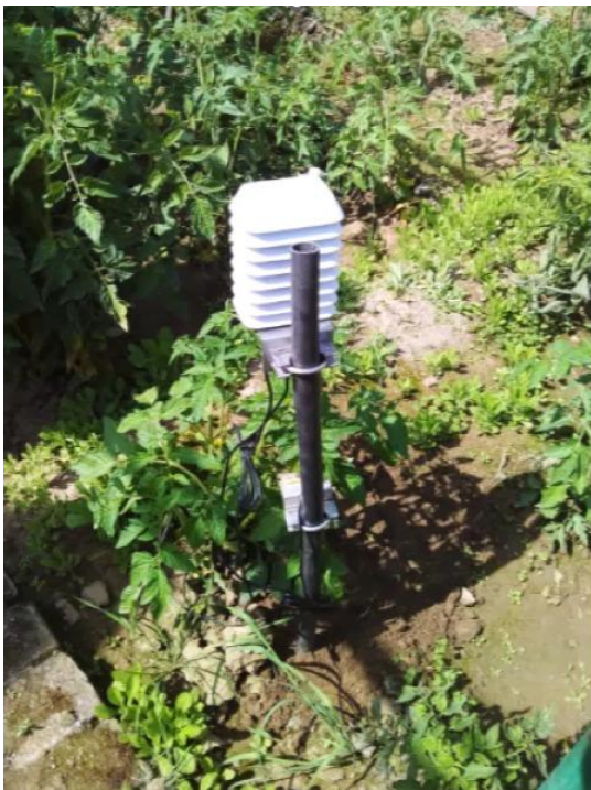
Figure 1 IoT Data Loggers for collecting sensors data in field
