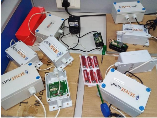
Figure 5. IoT sensor nodes prepared for testing and installation.
